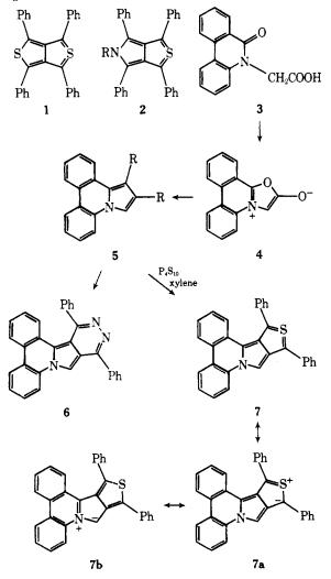
Trapping of the intermediate anhydro-2-hydroxyoxazolium hydroxide system 4 with acetylenic dipolarophiles is a convenient route to the ring system 5. Reaction of 4 with dimethyl acetylenedicarboxylate gave 5 ( $R = COOCH_3$ ) in 52% yield.
